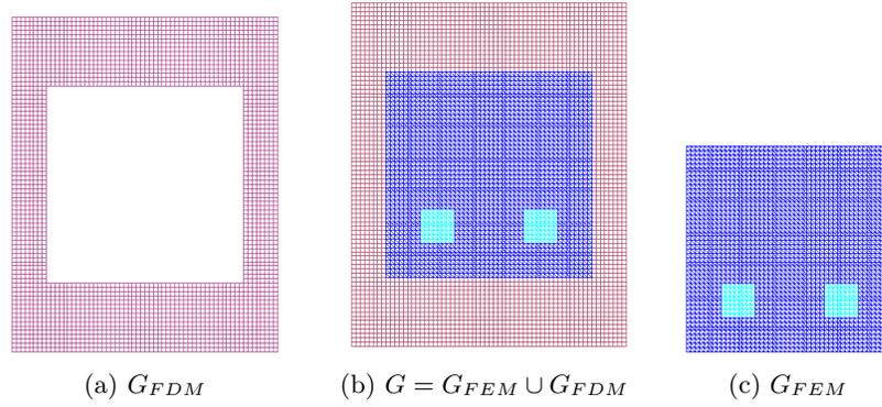
FIGURE 1. The hybrid mesh (b) is a combinations of a structured mesh (a), where FDM is applied, and a mesh (c), where we use FEM, with a thin overlapping of structured elements.
