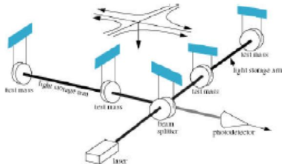
Fig-2: A schematic representation of the working of the Michelson-Morley Interferometers used at LIGO Hanford and Livingston. A source shines light on a beam splitter, which splits the beam into the “arms” of the detector. The test masses are suspended freely as a pendulum. The recombination usually results in no pattern, as the respective waves are out of phase. If a gravitational wave passes through the detector, there is an interference pattern observed.
